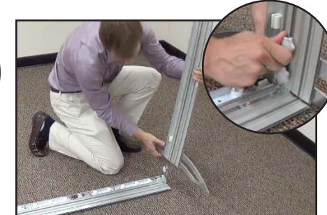
Slide extrusion assembly onto L-Bracket and tighten 2 thumb screws.
