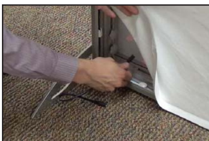
Peel back the bottom left corner of the backer. Remove LED connector from clip.
