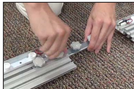
Insert CSS halfway into middle extrusion and tighten 2 thumb screws.
