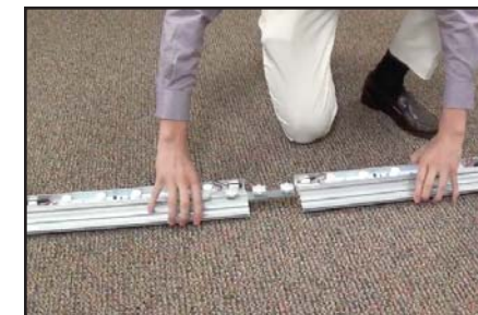
Connect middle extrusion and tighten 2 thumb screws.
