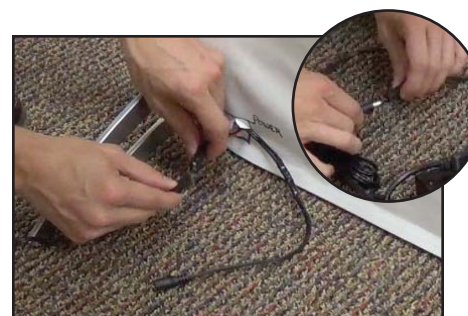
Connect the LED driver to the LED connector for the bottom row of lights and connect the other LED driver to the cord extension for the top row of lights.
