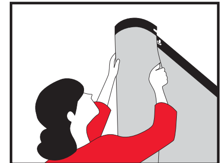
Bow endcaps and lift onto studs atop both sides of frame. For hinged panels hook one side then the other. Slide hands along length of panel to bond magnets.
