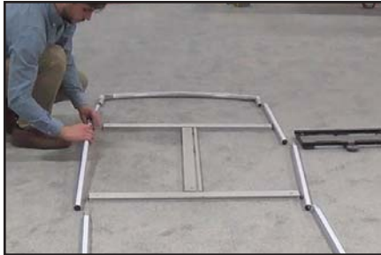
Connect the side tubes. Insert tube until button lock engages.
