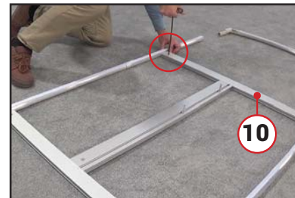
Insert part #10 into hole on the other side tube and secure CAM Lock using hex key.
