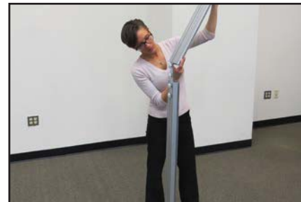
Connect second extrusion section onto CSS. Tighten 2 thumb screws.
