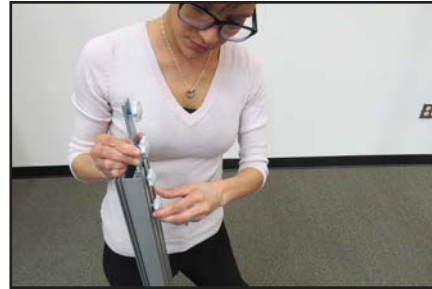
Insert CSS halfway into side extrusion. Tighten 2 thumb screws.
