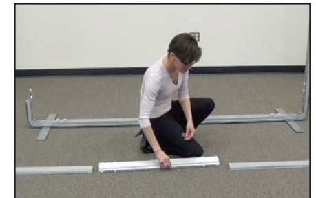
Lay out 3 extrusion sections of vertical support.
